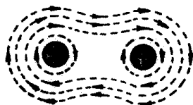
Fig. 1. FORCE OF ATTRACTION BETWEEN TWO PARALLEL CONDUCTORS
